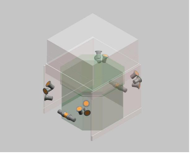
Figure 3-2: Placement of GBM Detectors on GLAST
