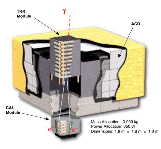
Figure 3-1: LAT Instrument Schematic
