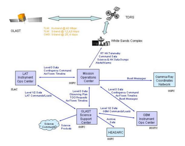
**Figure 4-1:** GLAST Ground Operations Overview. Only the elements involved in the data management during normal operations are shown.
